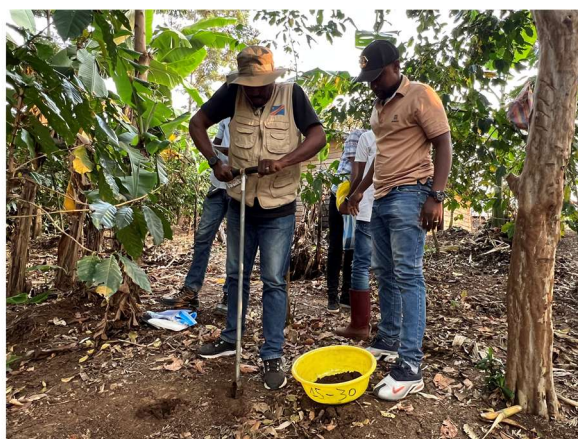
Figure 5. Soil sampling process using auger
