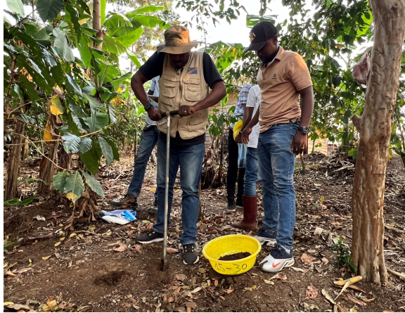
Figure 2. Soil sampling process using auger
